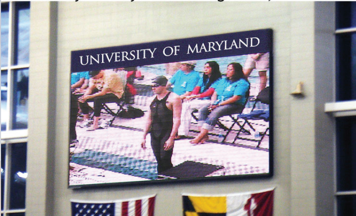
23mm Full Color Indoor LED Matrix Display (128 x 240) - 2.9m x 5.5m (10 ft x 18 ft)
