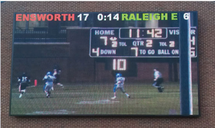
16.25mm Full Color Outdoor LED Matrix Display (300 x 520) - 4.9m x 8.5m (16.1 ft x 27.9 ft)
